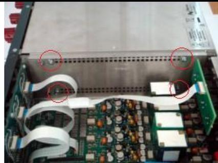
Replace the lid and replace the 7 screws to fasten it in place.
