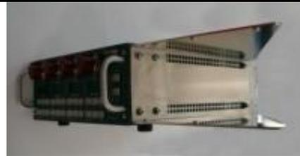
Fasten the large 19" mounting ear to the triangular strengthening plate using the 6x M3x6mm countersunk screws
