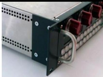
Mount the 4081 unit assembly into a 19" rack using suitable rack-mounting screws and connect all cabling to the rear of the unit. Remove the 4 feet from the bottom of the 4081 unit if required
