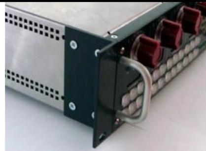
Mount the 2x 4081 unit assembly into a 19" rack using suitable rack-mounting screws and connect all cabling to the rear of the units. Remove the 4 feet from the bottom of the 4081 unit if required
