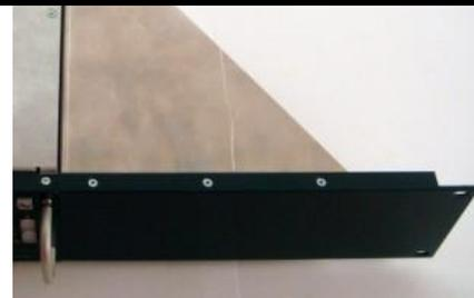
Fasten 1x small 19" mounting ear to the other side of the 4081 using 4x M4x6mm countersunk screws
